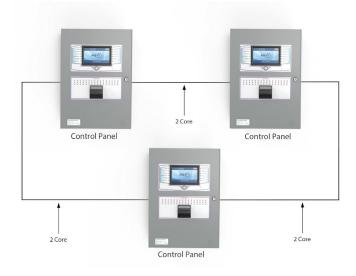
Two core loop wiring ensures network integrity by providing full isolation of faulty wiring segments.
