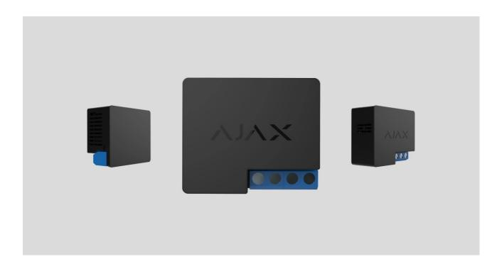
**Relay** is a dry contact relay to control a power supply remotely. The relay's dry contacts are electrically isolated to the power supply circuit of the device. Relay can be used in both low-voltage and domestic power grids. The device features two types of protection: voltage and temperature.
