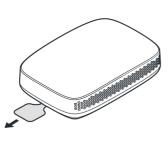
Pull the battery tab to activate the sensor
